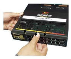
(2 each on top and bott0m and one each on the side). Remove these screws. Once these screws are removed, the front panel is easily slid out to the front of the chassis base.
